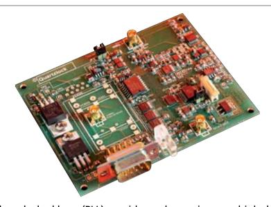
The A6-CPS digital phase locked loop (PLL) provides an low noise, very high short term stability filtered output which can be customised to a specific application. The A6-CPS digital PLL may be fitted into the Quartzlock A6 frequency convertor with BVA OCXO, rubidium, GPS or other options.
