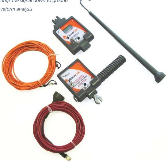
The Volt LiteWire is a medium voltage voltmeter designed for lines and substations. These units are designed for use with a hotstick and universal chuck adapter. The Volt LiteWire measures voltage phase to phase or phase to ground. It is a two-piece, True RMS voltmeter with a fiber optic link between the high voltage sensor and the readout at ground potential. The sensor is mounted on a hotstick and slipped onto a medium voltage line.
