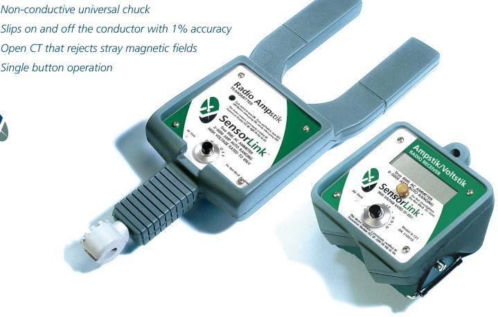
The Radio Ampstik uses the same current sensor technology as the original Ampstik. The key feature of this unit is the ability to display the current reading up to 50 feet away from the sensor. The user has the option to hold the display in their hands, mount it to a hotstick, or hang it on the
