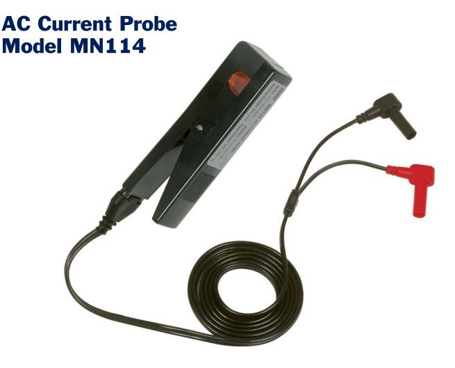
Small, compact and very tough, the Model MN114 is designed for measurements from 1mA to 10AAC. The "clothes pin" shape makes it ideal for use in tight areas, such as breaker panels, controller panels or outlets. They are excellent companions to all DMMs.
