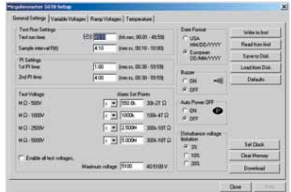
Four tabbed dialog boxes allow for clear and easy setup of all functions of the Model 5070, including setup for variable voltage and alarm set points, as well as step voltage tests and temperature compensation.
