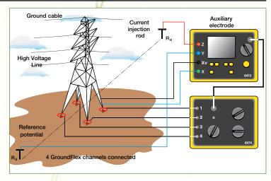
Used in conjunction with the Model 6474 vectorial processing unit, the Model 6472 offers the possibility of measuring a tower's ground resistance even if it is part of a parallel ground network, by selective measurement of the tower in question.
