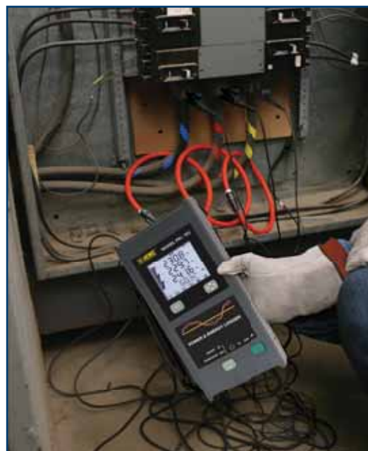
The backlit display on the Model PEL 103 can be read in dark areas showing the real-time measurements.
