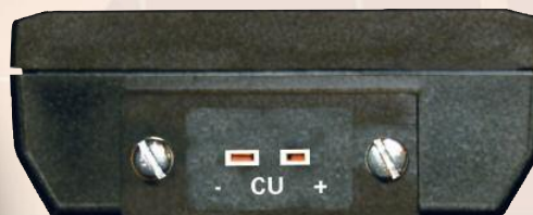
The TC-100 accepts both Mini-plug AND bare thermocouple wires
