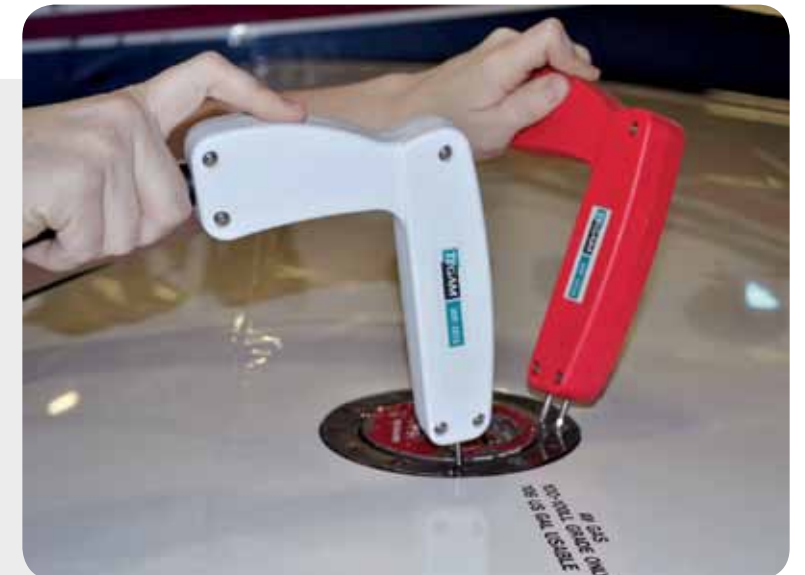
The HTP-101A pistol grip probes have hardened stainless steel pins that rotate on compression to break through oxides and paint where necessary.
