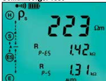
The Schlumberger test displays test lead connection, soil resistivity ( \rho ) test results, test electrode resistance and more.
