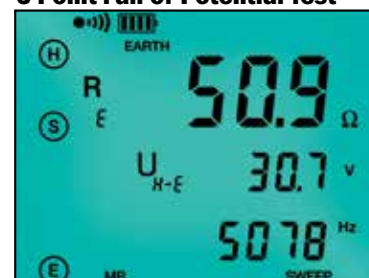
The 3-Point Fall-of-Potential test displays test lead connection, grounding electrode resistance, test voltage and frequency.
