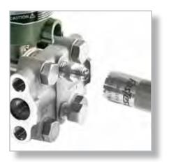
*FasTest* sleeve actuated *60 Series* connectors are ideal fast, safe and repeatable connections to a wide variety of thread used in process and manufacturing industries for filling, pressure and leak testing, and instrument calibration. Simply insert male threaded end into the connector and push the latching sleeve forward to complete the connection. Remove test pressure and pull back the latching sleeve to release the connection.
