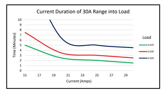
Measurement Conditions : Ambient Temperature 20'C, Mains Voltage 230V, Mains Frequency 50Hz Allow at least 7 minutes 'off' period between current output
