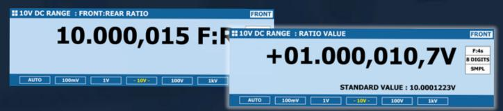
The 8104 comes fitted with electronically switchable rear panel inputs as standard enabling the 8104 to perform ratio measurements between two sources. Combined with exception linearity the ratio functionality can replace the use of Kelvin Varley Dividers in precision voltage measurement.
