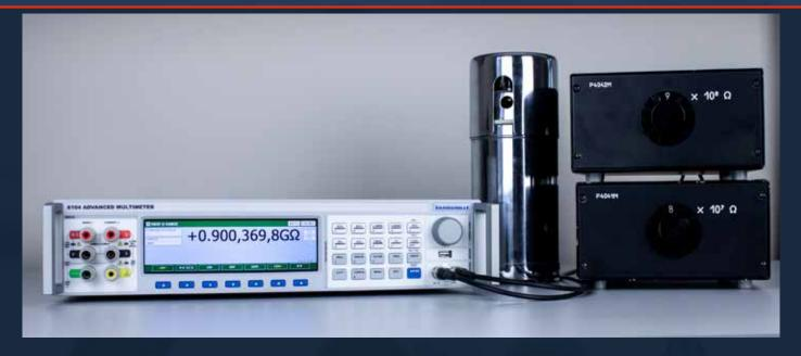
The dedicated electrometer input of the 8104 enables measurement of both low currents with resolution of 0.01pA and high value resistance in excess of 1 TOhm with exceptional noise performance and fast settling time.
