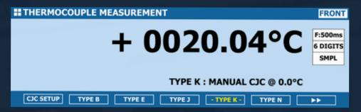
The 8104 offers direct thermocouple conversion to simplify measurement of thermocouples and thermocouple simulators. The 8104 dynamically displays the currently measured voltage as well as the conversion to temperature simultaneously for ease of use.
