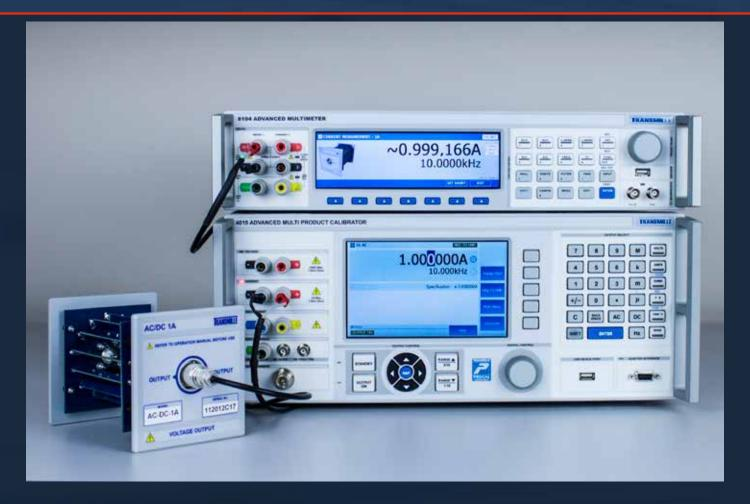
The 8100 Series has been optimised for use with Transmille's range of AC/DC current shunts enabling DC and offset parameters to be entered in providing direct measurement of applied current on the screen. The 8100 simultaneously measures the voltage and frequency and performs a real time correction based upon the AC/DC difference at the current frequency and the value of the shunt.
