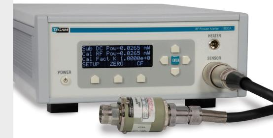
Thermistor RF power sensors are universally recognized as the most accurate means to measure and transfer RF power. The TEGAM Model 1830A was designed to operate with all types of thermistor RF power sensors while reducing uncertainties. It combines a modern DC substitution bridge with a precision measurement system to provide consistent, calibrated RF power readings manually or automatically.
