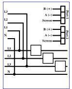
Self powered 3 Phase 4 Wire **Unbalanced** Load
