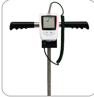
Fastening on stand with temperature data logger
