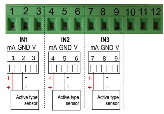
Connection of the0-5/10 V voltage inputs:
