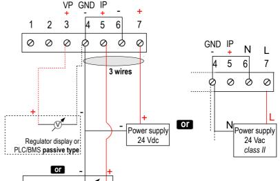
connect the output ground to the input ground. See drawing below.
