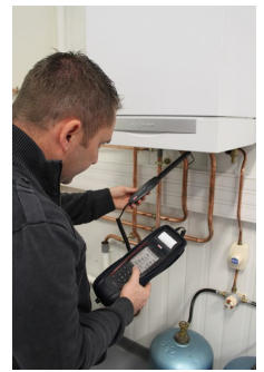
Ambient CO checking
