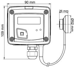
Material: ABS V0 as per UL94 Protection: IP65 Display: LCD 10 digits. Size: 50 x 17 mm Height of digits: Values: 10 mm; Units: 5 mm Cable gland: For cables Ø8 mm maximum Weight: 140 g Remote probe: cable of 2 m length in PVC
