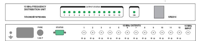
Ten indicators give the status of the outputs individually. If the signal is present at the output the indicator is green if not the indicator is red and it indicates the number of the broken down way.
