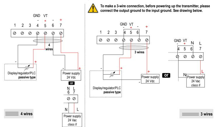
For TM110 - PO and TM110 - PN models with 4-20 mA output - passive :
